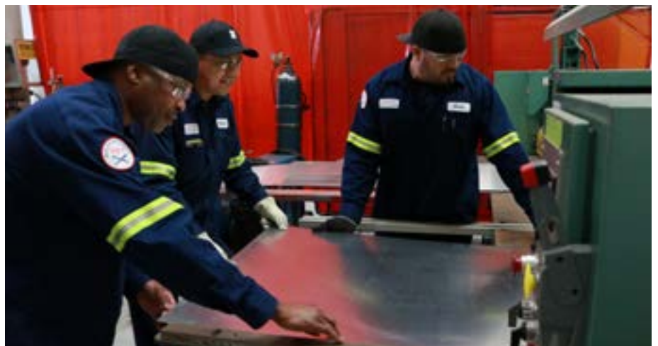
MTS Maintenance Mechanics Lawrence Gill, Arturo Avina, and Juan Ibarra run sheet metal through a shear as part of a bus repair project. (Photo was taken prior to social distancing/face covering requirements due to COVID-19 pandemic)
