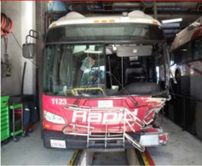
The Body Shop crew had to remove this Rapid bus' entire front end and rebuild it.
