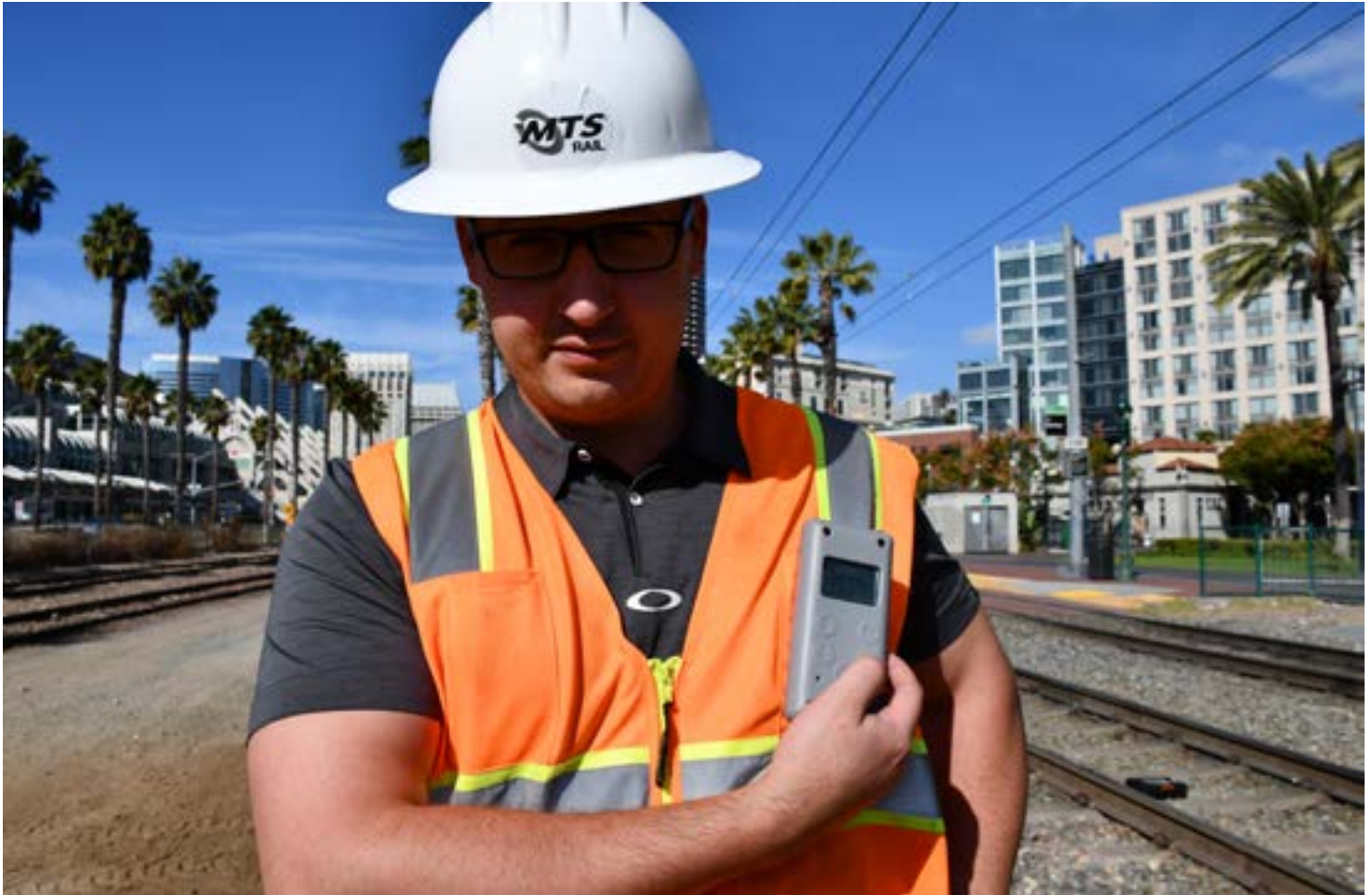
Transportation Supervisor/Controller Justin Wayne shows off wearable EWD equipment now used by track work crews. (photo taken prior to employee face covering requirement due to COVID-19 pandemic)
