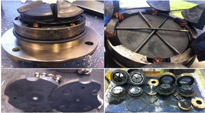
Figure 1 - Damaged Grounding Contacts
