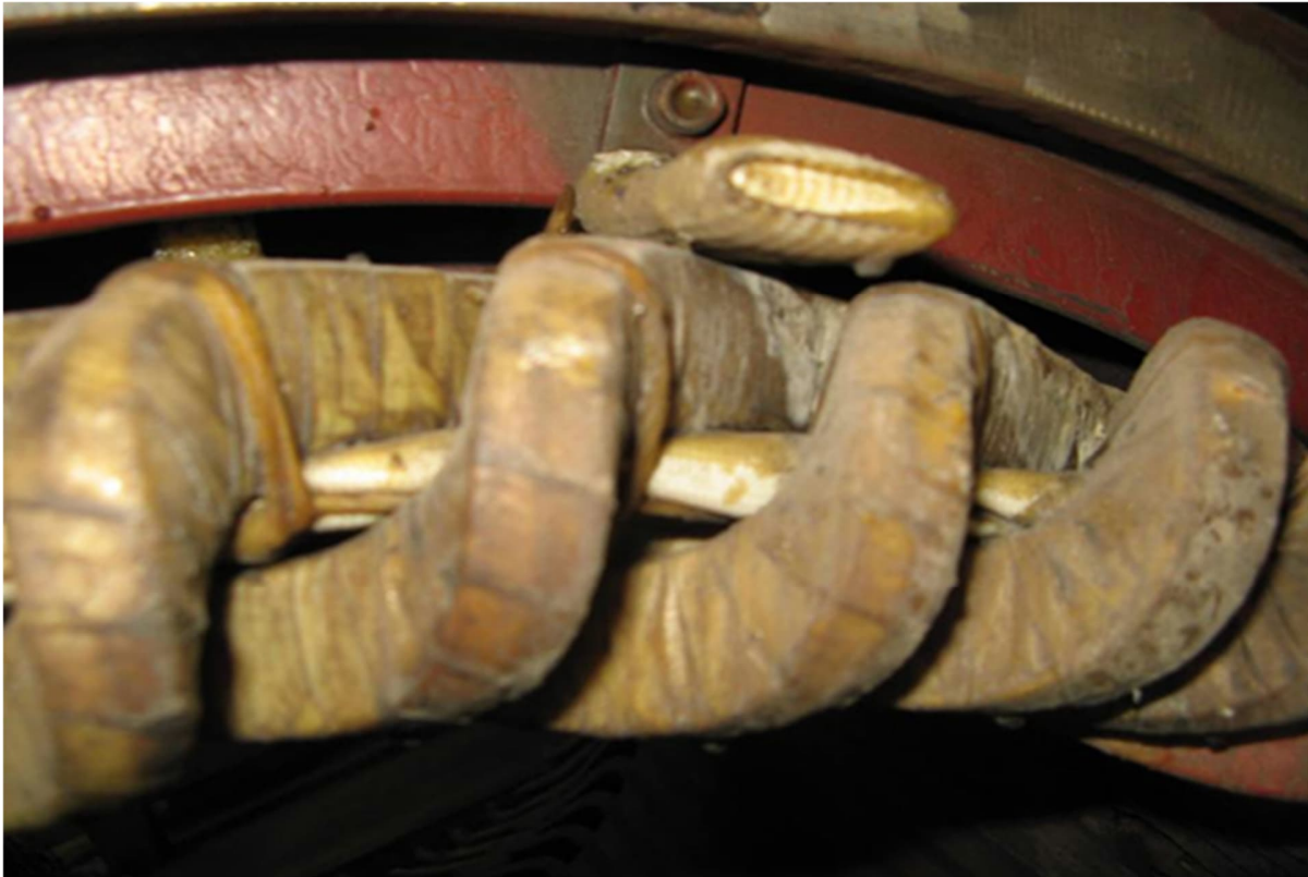
Figure 4 - Motor windings rewound by independent shop
