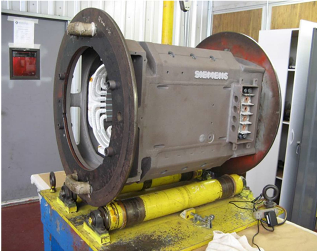
Figure 6 - Fixture to rotate the motor during cooling to prevent resin accumulation
